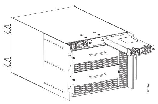
Figure 38. Removing and installing a power supply
